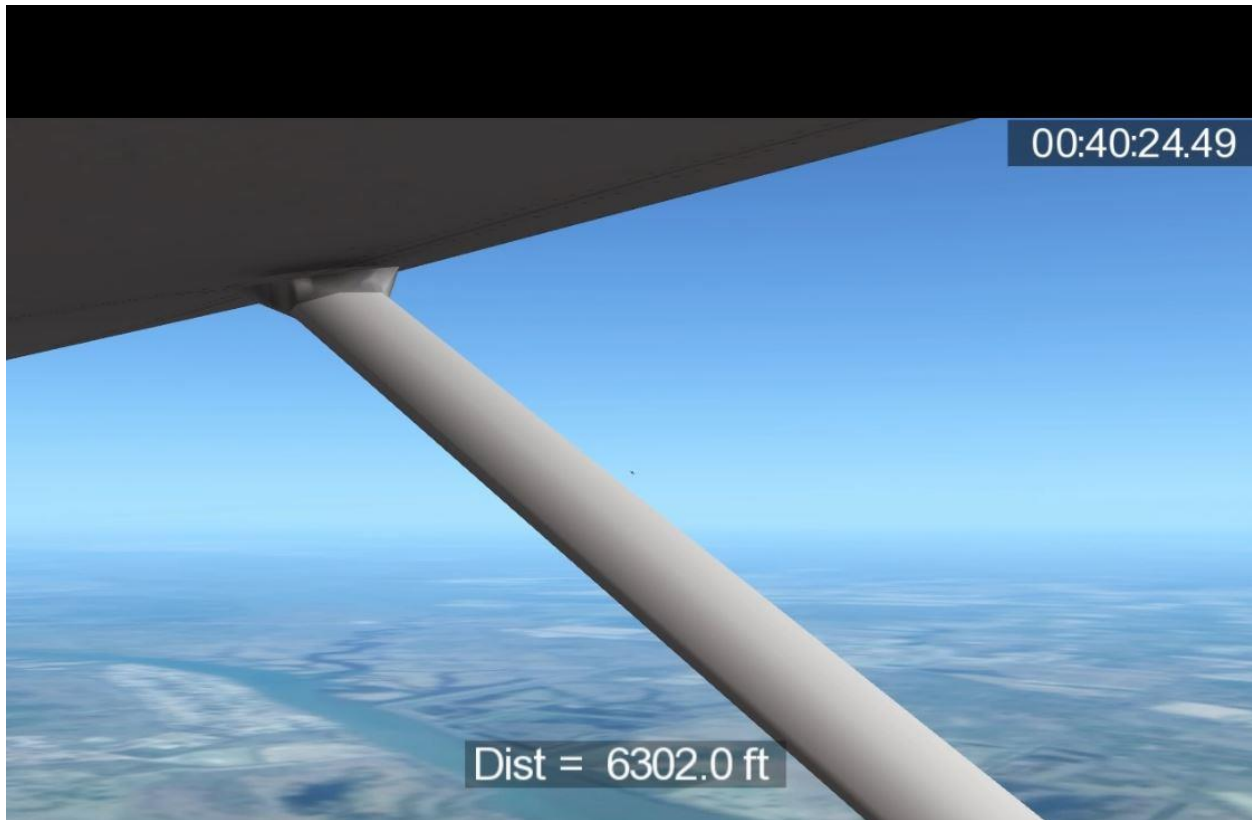
[Figure 9: Simulated view from MA2: MA1 appears in center of screen before becoming obscured by strut (Tab Z-19)]
